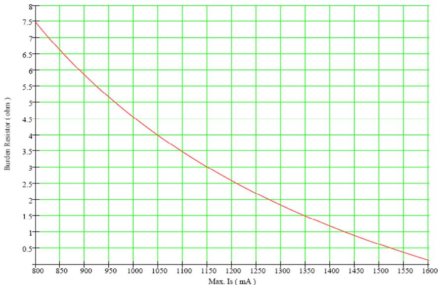
To maintain safe start-up  $R_M$  must not exceed 3 Ω during fault condition.
